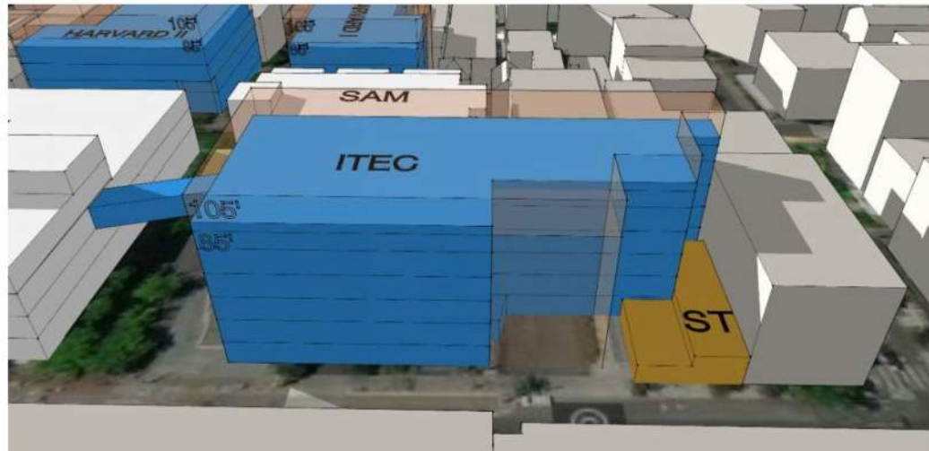
ITEC – Six stories and approximately 95 feet
