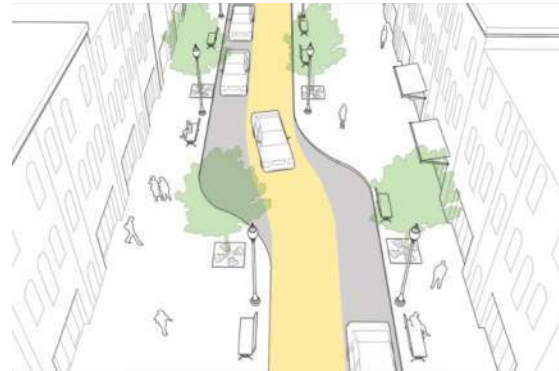
Traffic-calming chicane design from SDOT Streets illustrated.
