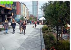
1. Continuous pavement with different colors 2. Planting beds minimize street, maximize sidewalk 3. Sidewalk and street at the same level 4. Festival street opportunity
