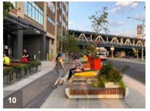
10 • Modular sidewalk furniture provides planter boxes and seating • Different pavement types create zones on the sidewalk
