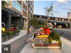
15 • Pavement types suggest different zones • Street furniture provides seating and planting beds • Street furniture is not integral/structural to sidewalk - is movable/changeable • Multiple small/medium scale furniture pieces can have different features
