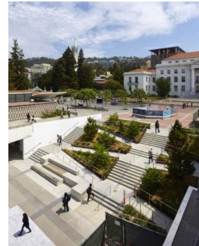
Use a combination of stairs & ramps to provide universal access on campus
