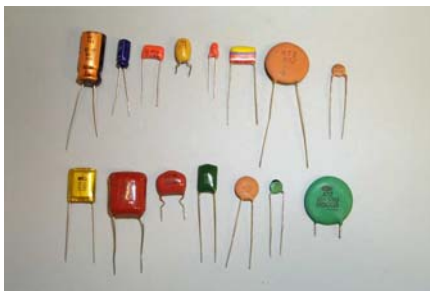
Figure 4 - Different types of capacitors. Ceramic disk capacitors are on the right in the photograph. The capacitor circuit symbol is on the right of the figure.
